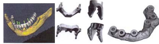
Gambar-12 Model Computer alat bantu penuntun bor bedah gigi (dental drilling guide) [Lorrison 2001]
