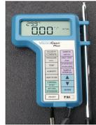
Gambar 6 Anemometer digital tipe Am-4240-Hot Wire Anemometer
