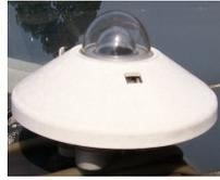
Gambar 5 *Pyranometer* tipe CC48
