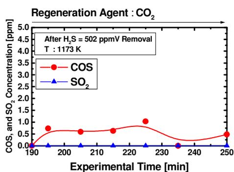
Figure 11 Result of Used MAC Regeneration Test following H<sub>2</sub>S Removal
