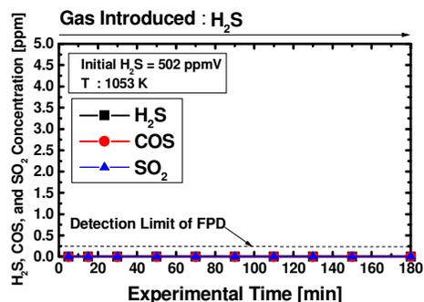
Figure 9 Result of H<sub>2</sub>S Removal at 1053 K
