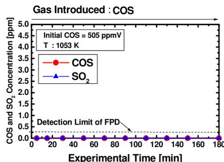
Figure 10 Result of COS Removal at 1053 K
