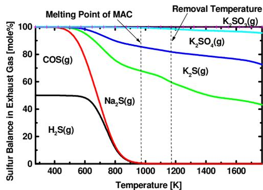
Figure 4 Chemical Equilibrium Calculation of Mixed Gases ( $H_2S+CO_2$ ) Removal
