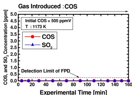
Figure 8 Result of COS Removal at 1173 K
