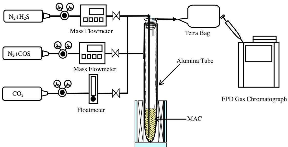
Figure 1 Experimental Apparatus for Removal and Regeneration Tests
