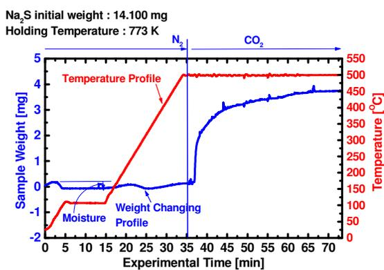
Figure 13 TG Result of Na<sub>2</sub>S Regeneration in CO<sub>2</sub>
