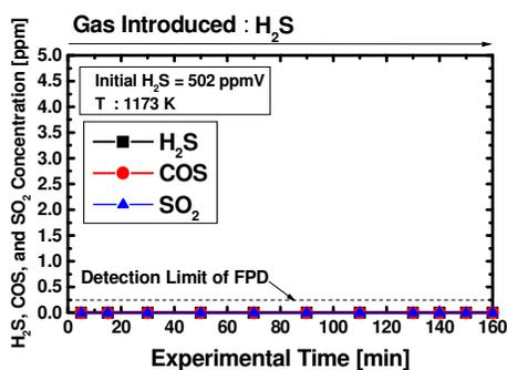
Figure 7 Result of H<sub>2</sub>S Removal at 1173 K
