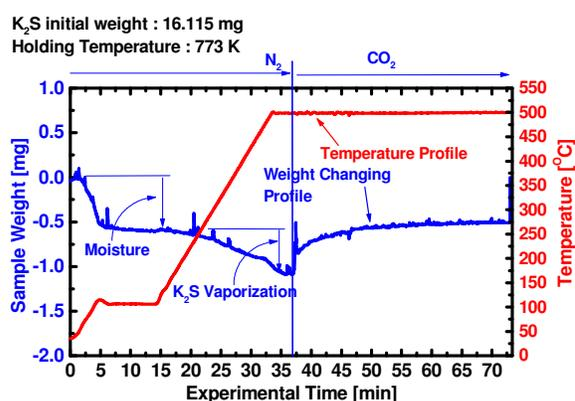
Figure 14 TG Result of K<sub>2</sub>S Regeneration in CO<sub>2</sub>
