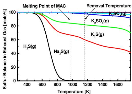
Figure 2 Chemical Equilibrium Calculation of H<sub>2</sub>S Removal
