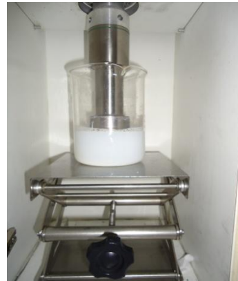
Diiradiasi ultrasonik selama 1 jam suhu 50 °C, P=200 watt
