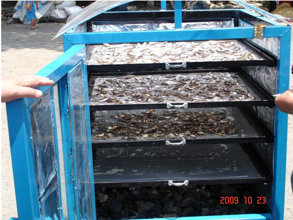
Figure 7. Drying machine by used the solar radiation from Sibermas Team with capacity 10kg/3 hr
